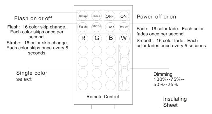
**Note:** When using the remote, please remove the insulating sheet. If you replace the insulating sheet when you are not using the remote, it will conserve battery power.
