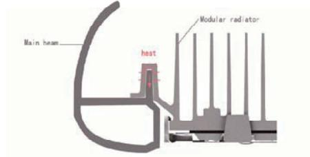
The heat is transferred to the main beam, and thus the main beam can promote the heat dissipation of radiator.
