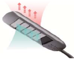
Schematic diagram of heat dissipation of honeycomb effect
